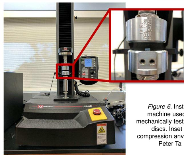
Figure 6. Instron machine used to mechanically test GelMA discs. Inset is compression anvil. P.C.: Peter Ta
