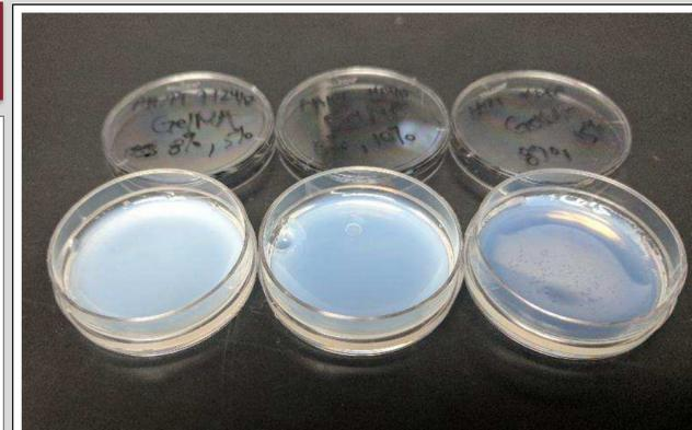
Figure 9. Different w/v samples of 8% methacrylation degree.
