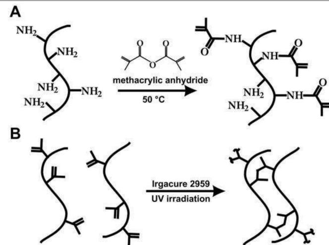
Figure 4. Binding of methacrylic anhydride to the gelatin and subsequent crosslinking by UV light creating final version of gel. P.C.: Nichol et al., 2010.
