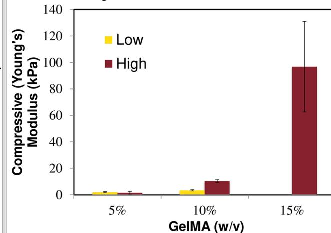
Figure 8. Compressive modulus for the different GelMA formulations. Note: we were unable to test 15% w/v of 0.25% degree of methacrylation because it did not properly crosslink.
