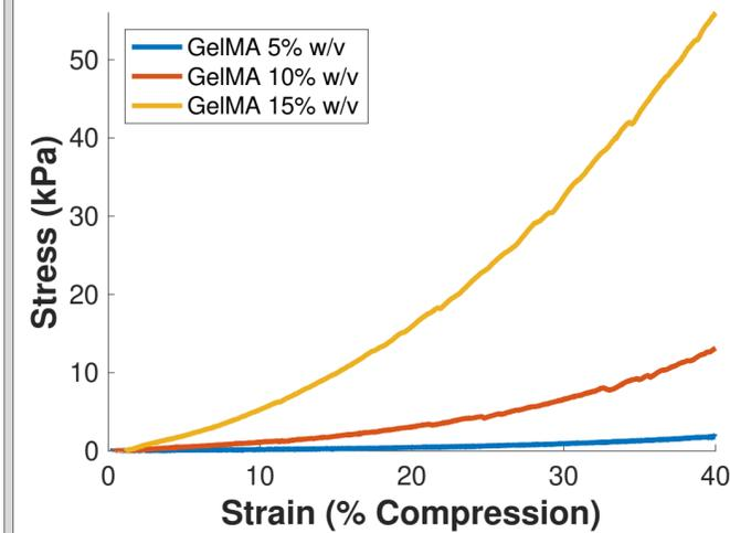
Figure 7. Stress vs Strain curve for different w/v ratios of the 8% degree of methacrylation batch.
