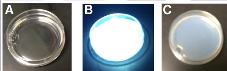
Figure 5. Process of crosslinking GelMA. (A) GelMA in pre-polymer solution. (B) Exposure to UV radiation. (C) Crosslinked GelMA hydrogel.
