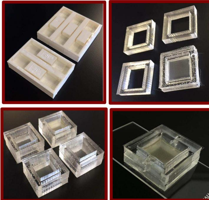
PDMS Window frames are made up of two PDMS windows, holding a mesh between them.
