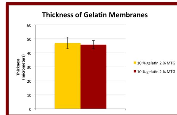
The error bars displayed are standard error, and The P value=.8, which means that the data was not statistically different, so therefore changing the percentage of MTG did not change the thickness of the membrane
