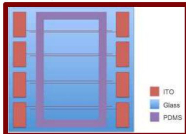
Bottom layer of the chamber would be glass, with tin oxide placed on the glass, so as to conduct electricity. The benefits of doing this is because the tin-oxide would be transparent, which allows the cardio-myocytes placed on the glass to be viewed
