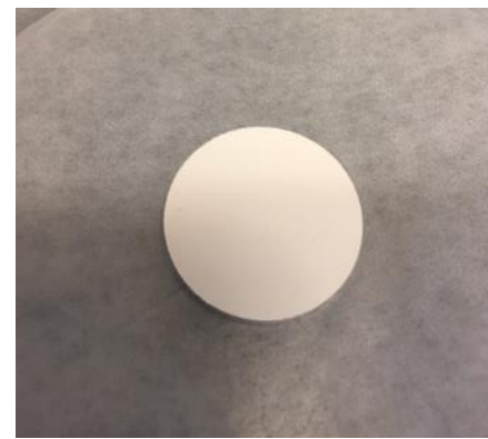
Figure 1b. SZO Pellet After Calcination. (PC: Shravan Hariharan)
