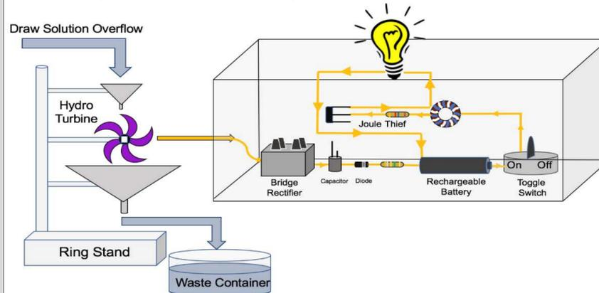
Fig. 4 Hydro-turbine and circuit schematic
