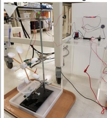
Fig. 5 Bench-scale hydro turbine for PRO bench-scale system
