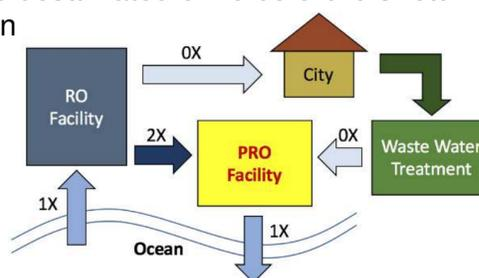
Fig. 3 Schematic of desalination with PRO
