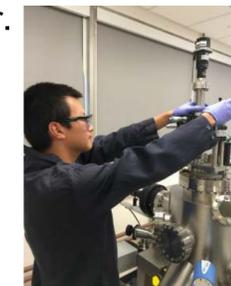
Fig 10. Adjusting the substrate position for ideal growth conditions. (PC: Thomas Orvis)
