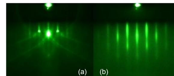
Fig 9 (a) Specular spot of the substrate before the PLD growth. (b) Diffraction pattern after 815 pulses, at the end of the PLD growth. (PC: Yizhi Huang)
