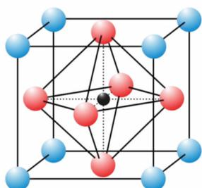
Fig 3. Unit cell of the BZO structure. It forms a general cubic shape similar to the typical perovskite structure. (PC: Haskel et al.)
