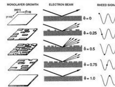
Fig 7. RHEED oscillation diagram. (PC: Neave et al, 1983.)
