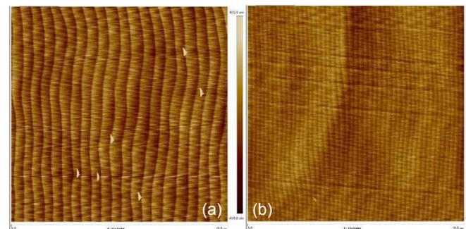
Fig 6. (a)  $\text{SrTiO}_3$  substrate before the growth. The vertical lines show 4 Angstrom high atomic steps. (b) BZO on STO after 25 unit cells of growth. Apparent atomic steps are observed showing it is a successful growth. (PC: Thomas Orvis)
