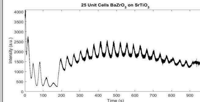
Fig 8. RHEED oscillations for my thin film sample. The oscillations can be counted to calculate film thickness. (PC: Yizhi Huang)
