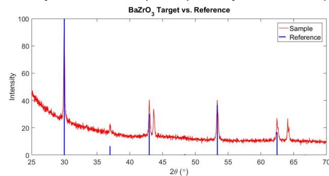
Fig 5. Based on thousands of data points from 25 to 70 degrees as 2 theta, I plotted this XRD graph using MATLAB and compared it to ICSD reference data. (PC: Yizhi Huang)
