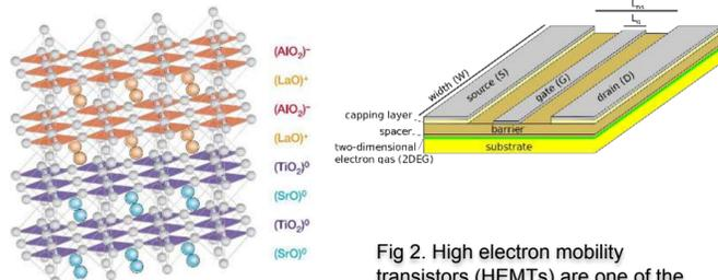
Fig 1. Schematic of the resulting (LaO)/(TiO<sub>2</sub>) interface. (PC: 2004\_NLett\_Ohtomo)
