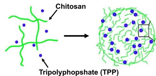
Figure 3. Formation of CS-NPs via ionic gelation (adapted from Chávez, 2011)
