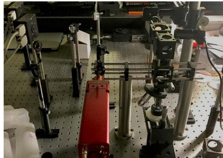
A photo of the micro-PL and Raman setup. Laser and white light enters the system onto the sample on the stage. PC: Sarah Moon
