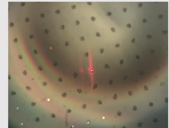
An image of a sample with 5 $\mu$ m radius InP dots and incident laser light taken by the camera using the 20X objective lens. PC: Sarah Moon
