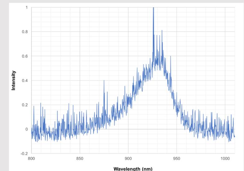
A graph of the PL from the same InP sample collected by the system using a 658 nm laser at 125 mA and 50 seconds of exposure. The bump around 920 nm is the observed PL.
