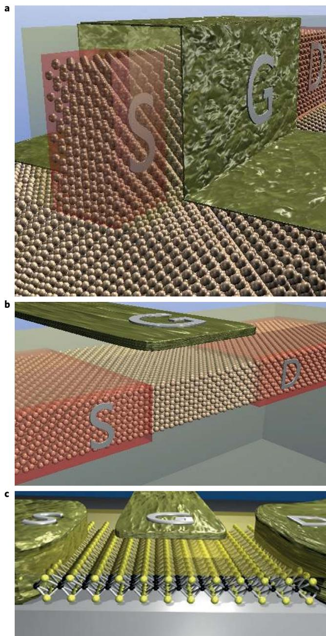
**Figure 1 | Sketch of new generation devices. a**, Tri-gate device. **b**, Ultrathin body device. **c**, 2DM-based device. In **a,b**, individual silicon atoms are visible at these length scales. In **c**, single-layer MoS<sub>2</sub> is the channel material. Doped source (S) and drain (D) are considered and highlighted in red in **a,b**, whereas metallic contacts are shown in **c**. The transparent yellow layer represents the oxide. Gate (G) is metallic.
