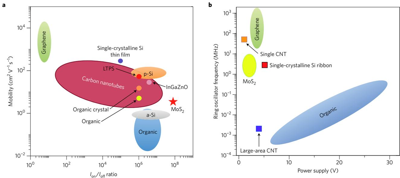
**Figure 5 | Figures of merit of transistors for flexible electronics. a,** Trade-off between  $\mu$  and  $I_{\text{on}}/I_{\text{off}}$  ratio for materials typically used in flexible electronics.
