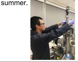
Fig 10. Adjusting the substrate position for ideal growth conditions. (PC: Thomas Orvis)
