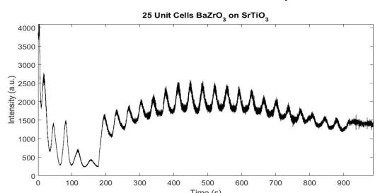
Fig 8. RHEED oscillations for my thin film sample. The oscillations can be counted to calculate film thickness. (PC:Yizhi Huang)
