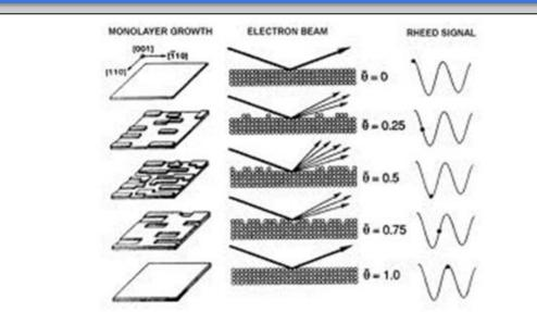
Fig 7. RHEED oscillation diagram. (PC: Neave et al, 1983.)
