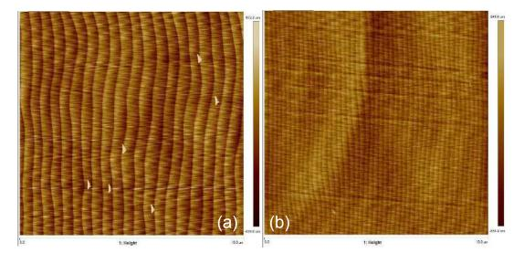
Fig 6. (a) SrTiO<sub>3</sub> substrate before the growth. The vertical lines show 4 Angstrom high atomic steps. (b) BZO on STO after 25 unit cells of growth. Apparent atomic steps are observed showing it is a successful growth. (PC: Thomas Orvis)
