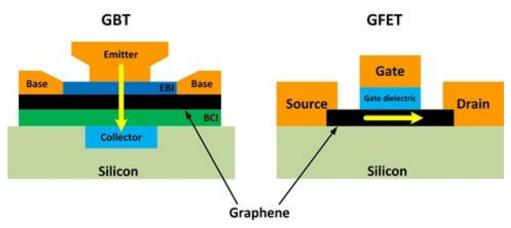
Two different methods of transferring current (data) via transistor
