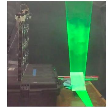
Using PIV to visualize a shear pattern, with the top rows of fans blowing harder than the bottom rows. PC: Sarah Fry
