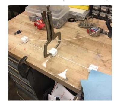
The parabolic support being glued to the acrylic sheet. The alignment blocks are the small white squares. PC: Brody Bishop
