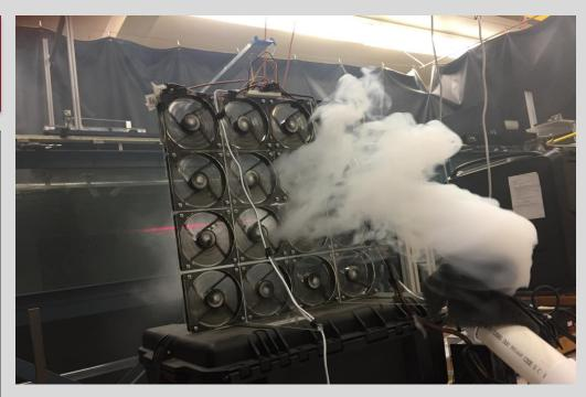
Testing the fan array using a smoke machine and the LDV
