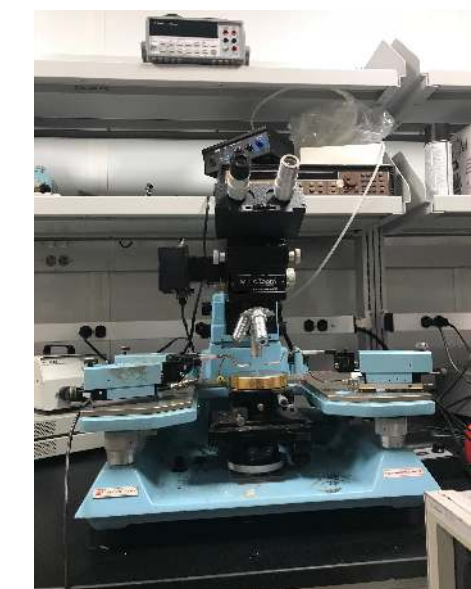
Figure 6. Probe station used for measuring devices. PC: Jessica Chao
