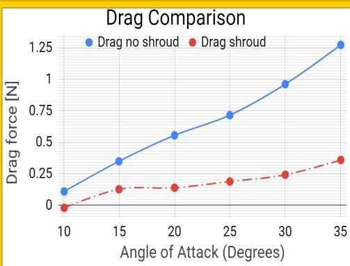
Evidently, the drag of the shrouded apparatus was significantly lower than the bare apparatus. The drag force was reduced by 70% when tested at speeds of 35 m/s.
