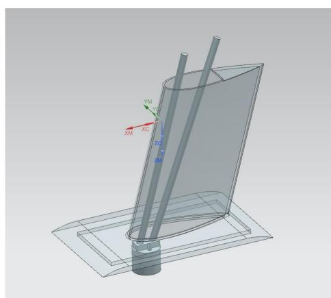
CAD design of the shroud and the setup
