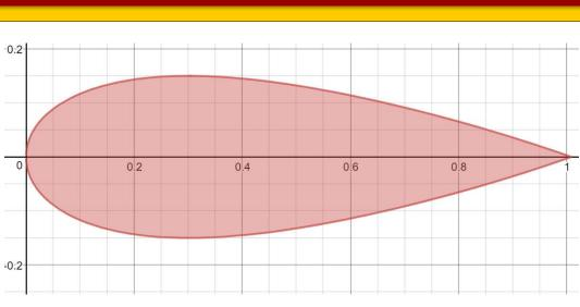
NACA 0030 airfoil, 0.3 units thick and 1 unit chord length
