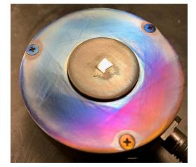
*Figure 2a.* VO<sub>2</sub> thin film on STO substrate. (PC: Oscar Chou)
