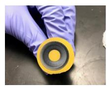
*Figure 7*. V<sub>2</sub>O<sub>5</sub> target after deposition (PC: Oscar Chou)
