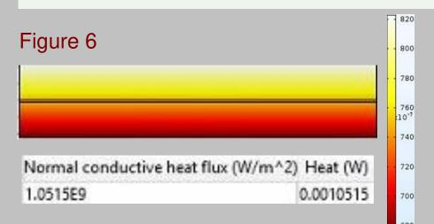
Temperature map of the Silicon Dioxide, Gold reflector heat barrier with derived numerical values for heat and heat flux
