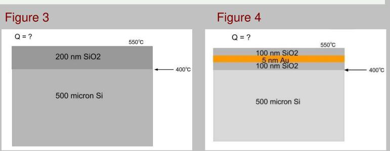
The first configuration of the heat barrier: a layer of Silicon Dioxide over a slab of Silicon.
