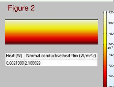
The second configuration of the heat barrier including a Gold reflector in between two Silicon Dioxide layers.
