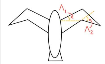
By cutting the wings of foam gliders, six different wing configurations were created with varying inboard and outboard sweep angles. The surface area of the wings were preserved across all six gliders.
