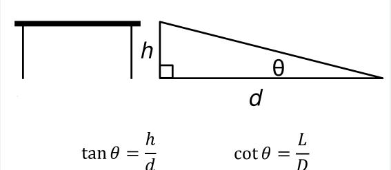
By measuring the horizontal distance flown (d) and change in height of the glider (h), the glide angle  $(\theta)$  can be determined. Using trigonometry, the lift to drag ratio (L/D) can be calculated.
