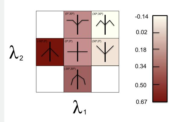
The diagram above depicts the six various wing configurations positioned by their respective inboard and outboard angles. The color gradient illustrates the static margin value for each glider wing. The graph below shows the average L/D for two different speeds tested on the wings.
