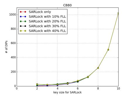
Fig.3 SARlock + FLL Implementation The number of DIPs is a good parameter to see the SAT resilience of the circuit. It is exponentially proportional to the key size of SARLock.
