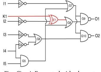
Fig.1 Circuit Encrypted with a key gate Inserted
