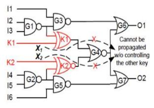
Encrypted circuit. This technique prevents sensitization as both Key-Gates,(K1 & K2), are parallel to each other. This brings difficulty to the attacker because they need to find the value of one key gate(K1), however, they need the value of the other key gate(K2) in order to find the first key gate(K1). But, they can't have the value of (K2) unless they have the value of (K1), and vice-versa. This technique is vulnerable to an attack, known as SAT-Attack.
