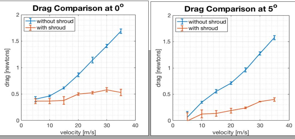
Figure 4: Results of Testing. It can be concluded that our shroud definitively reduced the drag of the apparatus. PC: Manaeha Rao.
