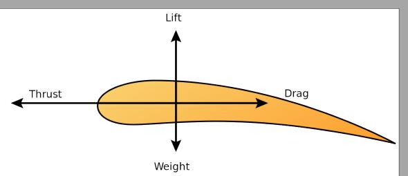
*Figure 1*: Aerodynamic Forces. These four forces act on all aircraft. <https://en.wikipedia.org/wiki/Aerodynamic force>
