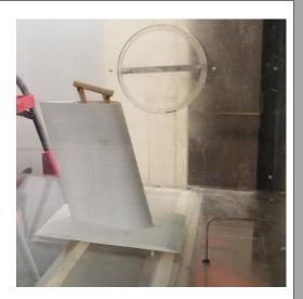
Figure 7: Shroud over apparatus. Our proposed solution was an aerodynamic shroud that would encompass the two cylinders to reduce their drag. We tested the drag of the apparatus with the shroud on top. PC: Saakar Byahut.
