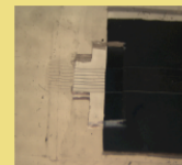
Figure 9: One of our PEG block models. We desired a slower melting rate for the PEG, thus we attempted to split the block into thirds. PC: Ahuva Weltman
