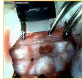
Figure 7: Insertion of our probe into a live rat. Probe was positioned carefully above insertion zones. We were careful to avoid contact between the insertion tool and cranium. PC: Ahuva Weltman, Leo Siow
