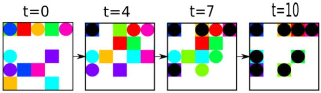
This example is our second step of multi agent path finding with many agents in a confined space. The colored squares indicate the robots and the corresponding circle is the goal it must reach. T indicates the time step.
