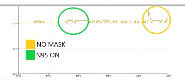
This graph of airflow measured from the spirometer shows the importance of wearing a mask amidst COVID, the use of which significantly decreases the output of airflow volume.
