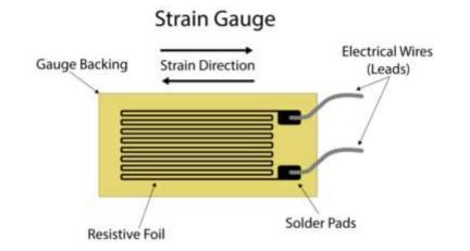
Figure 2. Piezoresistive Sensor, sensor attached to mesostructure able to read forces applied by displaying as change in electric current, Michigan Scientific Corporation
