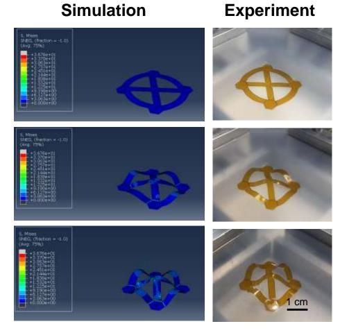
Figure 4. Abaqus simulation compared to real life images of a 3D structure formed by compressive buckling based on design in Figure 3, Amado Ochoa
