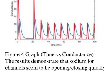
channels seem to be opening/closing quickly in comparison to the slower potassium ion channels, reinforcing the influx of sodium ions in the cell. Adapted from "Introduction to Computation Modeling: Hodgkin Huxley Model" by Andrew Jahn
