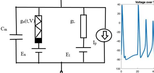
Figure 2. The basic diagram of the Hodgkin Huxley model displays an electrical representation of the biological neuron. PC: Josh Ok
