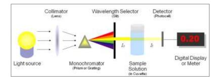
Figure 4. Spectrometry measures a substance's absorbance by passing a certain wavelength of light through it. PC: Chemistry LibreTexts
