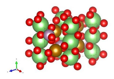
This is a full model of the compound structure called "LiFePO<sub>4</sub>"
