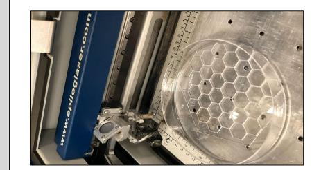
Create the cover slip by taking a petri dish and laser cutting it into hexagons
