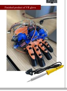
After all the hardware was put together, we inspected an Arduino Code from GitHub and tested out the potentiometers on the glove.
