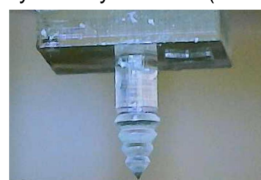
Fig 4. Microscopic picture of barbed microneedle in force sensor fixture
