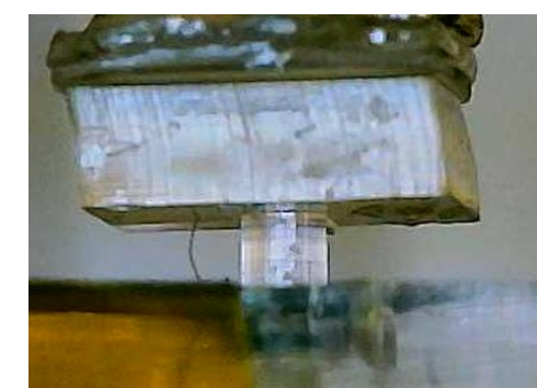
Fig 5. Microscopic picture of barbed microneedle inserted in PDMS
