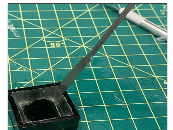
Figure 4: Cutting PDMS out of a 3D printed mold using a blade and scalpel. PC: Gianna Anguiano
