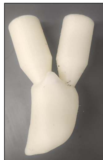
Figure 2: Left Ventricle 3D printed mold
